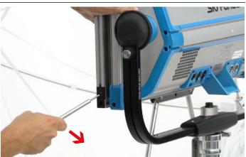
5.) It helps if you gently push the rods to the back of the housing so they slide easily into the Rabbit Ears insert hole.
