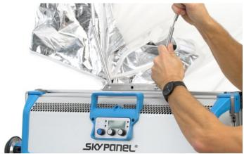
4.) With the Lantern hanging down you can start to install the other poles into the Rabbit Ears clockwise or counterclockwise.
