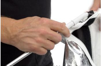
5.) Pull the rod extension 2 cm back into the elastic loop
