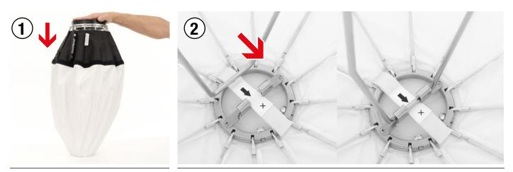
DOME instructions: Put the DOME on an even surface and push it down as shown in picture 1. By pushing the DOME down, the internal steel-stirrup approaches the two metal hooks as shown in picture 2. Make sure the steel-stirrup slides into the two hooks. In order to fold up the DOME, please push it down again and slide the steel-stirrup out of the two metal hooks.
